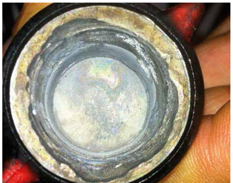
Fig 2 (right): Typical level of connector corrosion in a battery formation department
