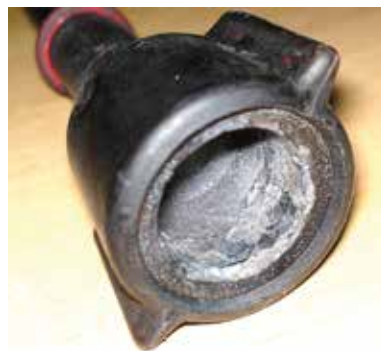
Fig 4: Used connector showing corroded and pitted internal contact surface.
